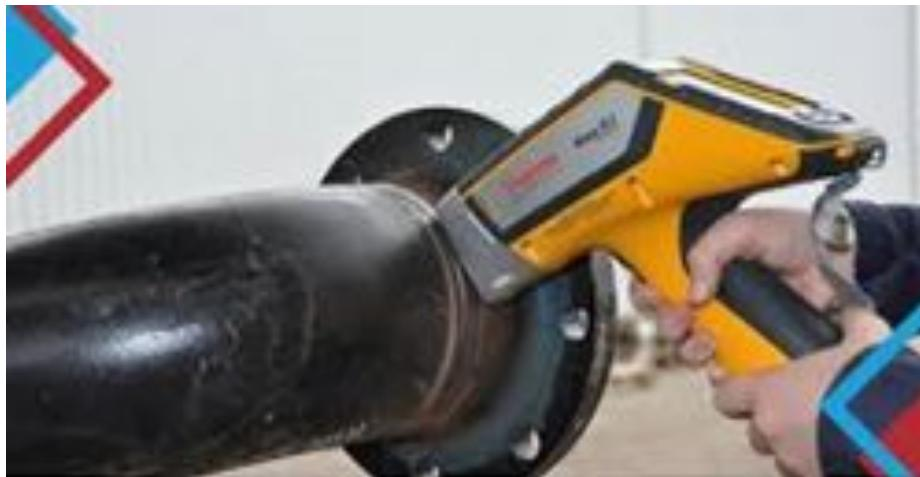
PMI (Positive Material Identification) testing is the analysis of materials to determine the chemical composition of a metal or alloy at particular (usually multiple) steps of alloy manufacturing or in-process alloy installation.
