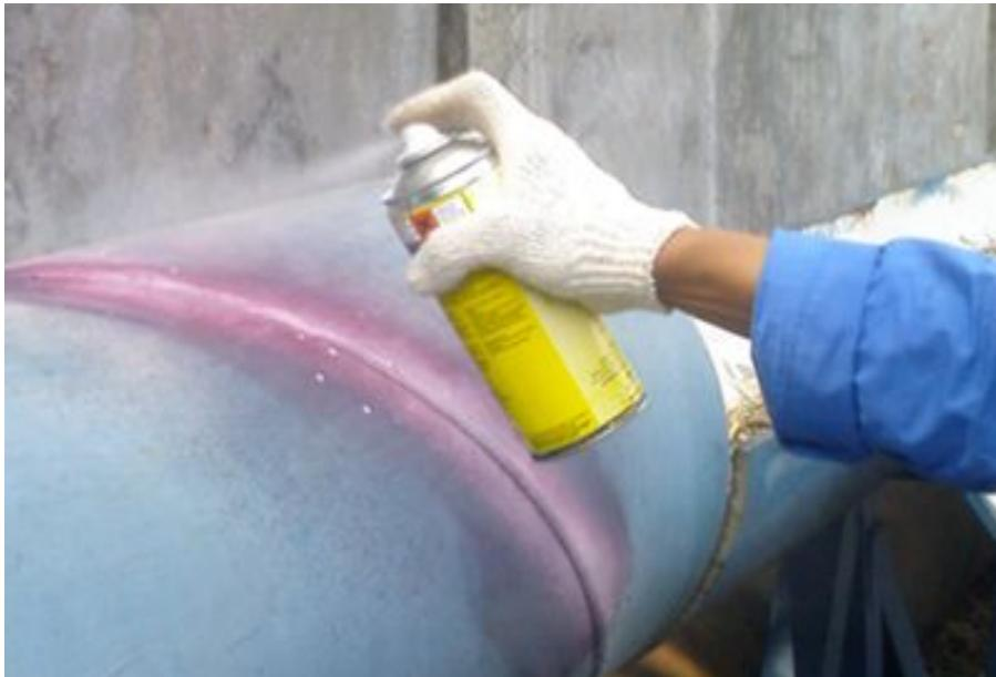
Liquid penetrant testing a widely applied and low-cost inspection method used to locate surface-breaking defects in all non-porous materials (metals, plastics, or ceramics).
